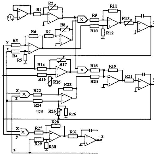
Figure 3. Circuitry realization of the unified hyperchaotic system (3). Resistors ( $k\Omega$ ):  $R3, R4, R5, R6, R9, R10, R11, R12, R18, R19, R20, R21, R23, R28, R29, R31 = 10, R1 = 2, R2 = 6.99, R7, R14, R15, R22, R27 = 1, R8 = 14.29, R13 = 3.80, R16 = 36.3, R17 = 59.2, R24 = 3.3, R25 = 1.487, R26 = 0.172, R30 = 0.288$ ; Capacitors ( $nF$ ):  $C_1, C_2, C_3 = 1$ . Op-Amps (1) (12): TL084; Multipliers: AD633.
