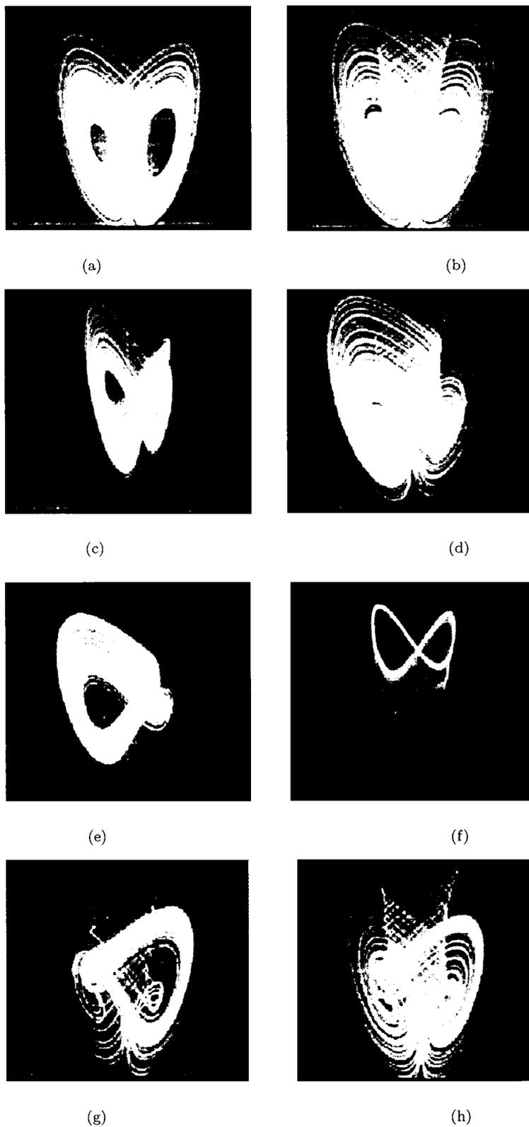
Phase portraits of the unified chaotic system (1) measured with the experimental setup in the  $x - z$  plane: (a) Lorenz-like attractor; (b) Chen-like attractor; (c) Lü-like attractor; (d)–(h): transition process. The scales of both vertical and horizontal axes are 0.2 V/div. The supplies of all active devices are  $\pm 14$  volts. The frequency of controlling signal is 0.5 Hz.
